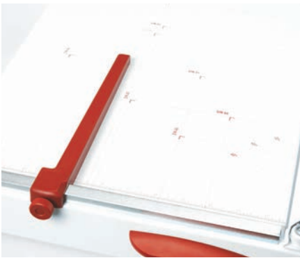
ADJUSTABLE BACK GAUGE Slide the back gauge to the desired position as indicated on the scale, then tighten knob to set.
