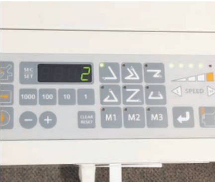
HIGH PROGRAMMABILITY In addition to 6 standard folds, the 1800S is capable of storing up to 30 custom programs in memory.
