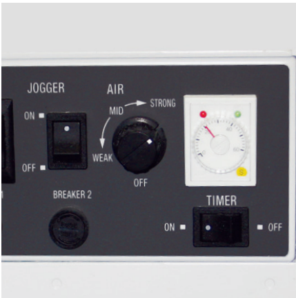
AUTOMATIC TIMER (AJ700) The timer function allows the operator to attend to other jobs while paper is being jogged.
