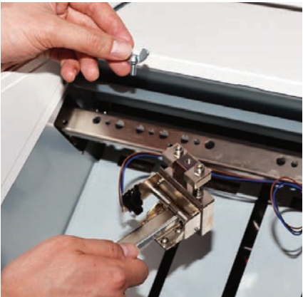
SETTING WITHOUT ANY TOOLS The iBOOKLET requires no tools to change staple head locations. Stapler head locations can be chosen from 5 slots.
